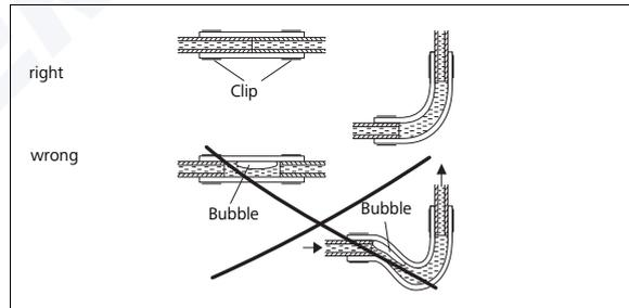
Fig. 13: Pipe/hose connection
