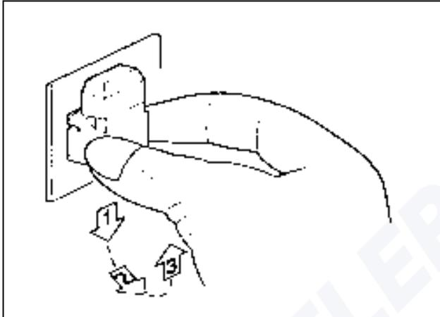
Fig. 23: Removing mounting plate on fuse holder
