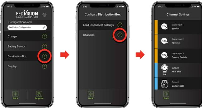
The Channel Settings page allows you to customise each of the connections to your RedVision Distribution Box. Simply put, you can tell RedVision what you have connected to it, and how you want RedVision to control that channel.
