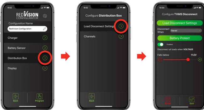
The 'Configure TVMS Disconnect' page allows you to set the Disconnect Triggers for the RedVision system.
