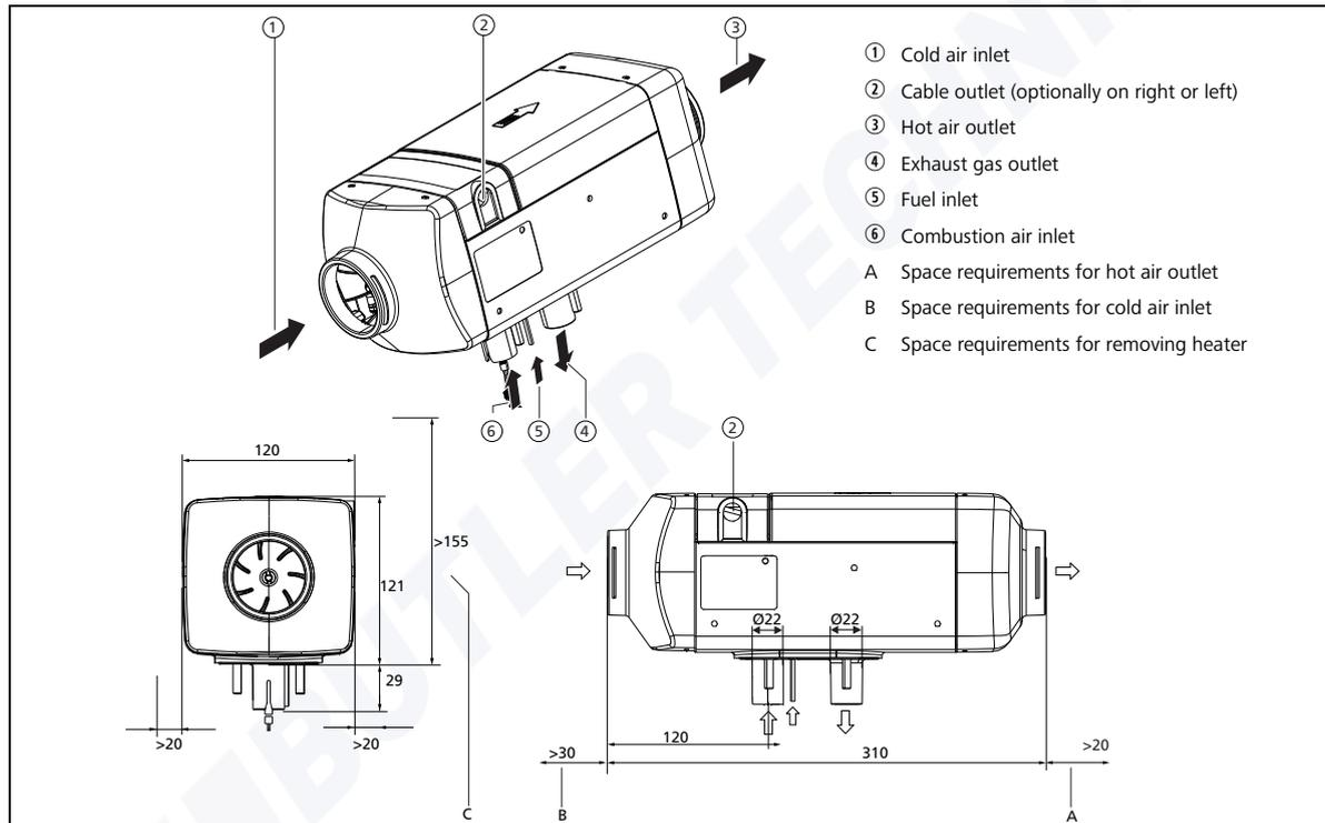
Fig. 1: Heater dimensions
