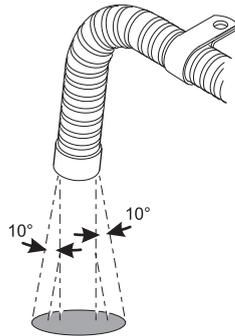
Outflow direction almost vertical  $90^\circ \pm 10^\circ$
