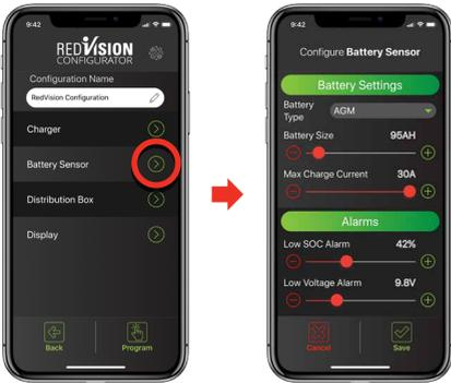
The Configure Battery Sensor page allows you to set the Battery Type, Size and Maximum Charge Current along with SoC and Voltage alarm levels.
