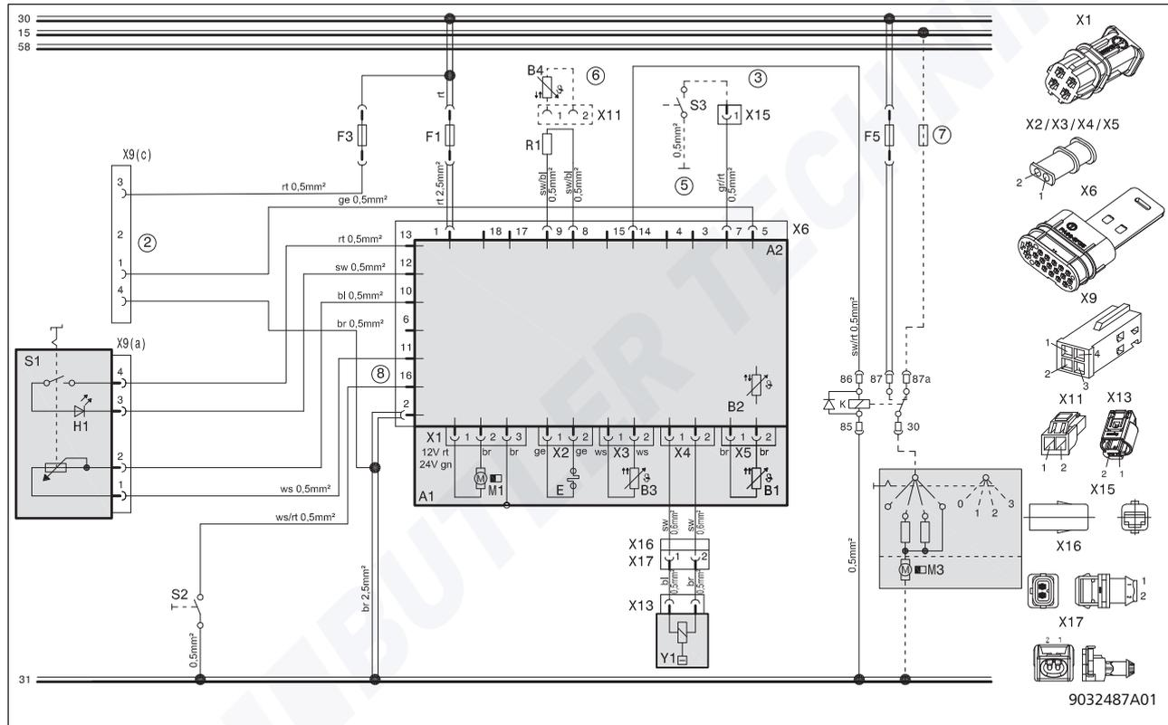
Fig. 29: System wiring diagram Air Top 2000 STC, 12 V/24 V with control element and vehicle fan, see Page 70 for legend
