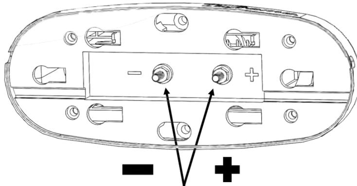
Attach corresponding wires here
