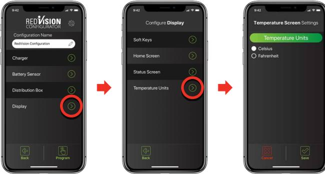
The Temperature Screen Settings page allows configuration of the RedVision Display Temperature Units. Select if you would like your units displayed in Celsius or Fahrenheit, then select Save.
