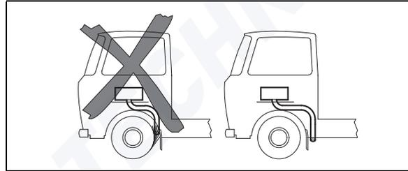
**Fig. 20: Prevent pipes becoming clogged with dirt**
